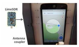
In the picture above a cheap LimeSDR is set-up with opensource software to transmit fake signals into the GPS of a mobile phone, making it believe that it is on Mount Everest.
