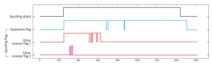
Three different receivers and their spoofing flags are shown. It is clear that the Septentrio receiver at the top is the only one with a trustworthy flag, which gives sufficient notification to the system about the spoofing attack. Warning: Heuristic algorithms based on insufficient amount of data are prone to overreact and set false spoofing flags, disturbing system operation.
