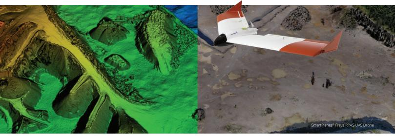
GeoTagZ enables a revolutionary new way of surveying. Used in combination with the AsteRx-m2 UAS or AsteRx-m2a UAS receiver it's now possible to achieve centimetre-level RTK ground precision from aerial survey. Using UAVs dramatically reduces time and cost in comparison to traditional ground survey.
