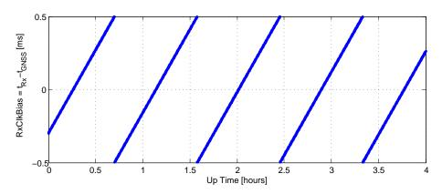
**Figure 2-1:** Example of the evolution of the receiver time offset with respect to the GNSS time in free-running mode.
