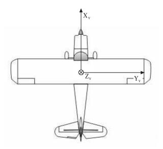
Figure A-1: Vehicle reference frame.
