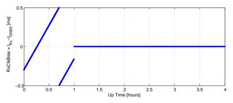
**Figure 2-2:** Effect of clock steering on the clock bias (clock steering enabled at an up time of 1 hour).
